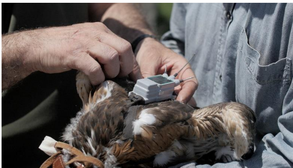
The E-OBS GPS-tag, model Solar 48G being fixed on eagle shoulders
